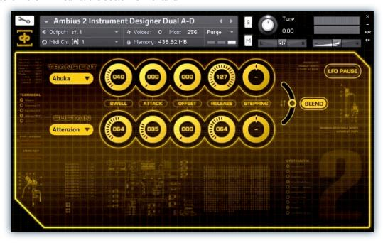
Each layer in Ambius 2 presets have individual controls for basic sound-shaping and performance adjustments. Each is also bound to a different midi CC to allow for easy automation.
