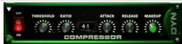
**Release knob** - This controls the release speed once signal drops below the threshold.
