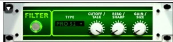
**Resonance/Sharpness knob** - This controls the amount of resonance added at the cutoff or peak node.
