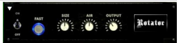
**Air** - Use this knob to adjust the simulated distance between the speaker and the microphone.
