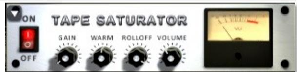
**Volume knob** - This knob controls the overall output level.
