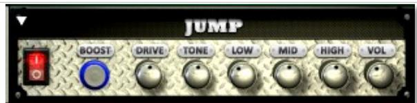
**Low, Mid & High knobs** - These control the low, mid and high frequency gain.
